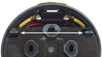
Once the keypad is in place, fasten it with one of the long machine screws provided. One is a standard phillips head. The other is a one-way design, making it difficult to remove. Use this screw only if your security needs require the keypad to be difficult to remove from its base, once installed.
