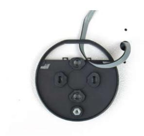
Note where the cable has been placed through the large opening at the top of the base. Fasten the base to the front of the safe, using the machine screws provided. The silver colored screws are 8-32, and the bronze colored screws are M6. Use whichever set is appropriate for the holes provided in the safe door. Discard the remaining set.
