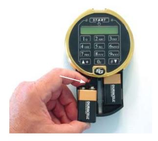
Place each battery into its section of the compartment as shown. Be careful to avoid scraping or binding the battery wires.
