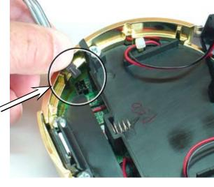
Place the battery compartment in the underside of the keypad. Note that the guide post is in the slot which is centered in the compartment. Each battery cable is routed through the top of the compartment—one on the left and one on the right. Make sure the battery wires do not get bound around the keypad's mounting feet or in the spring.
